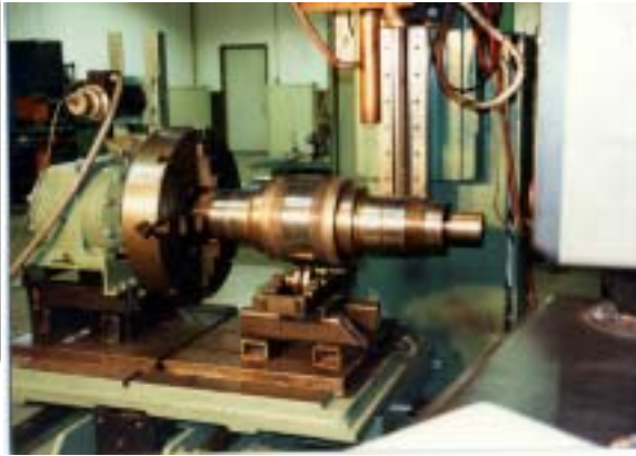
Mill shafts laser hardened bearing seat
