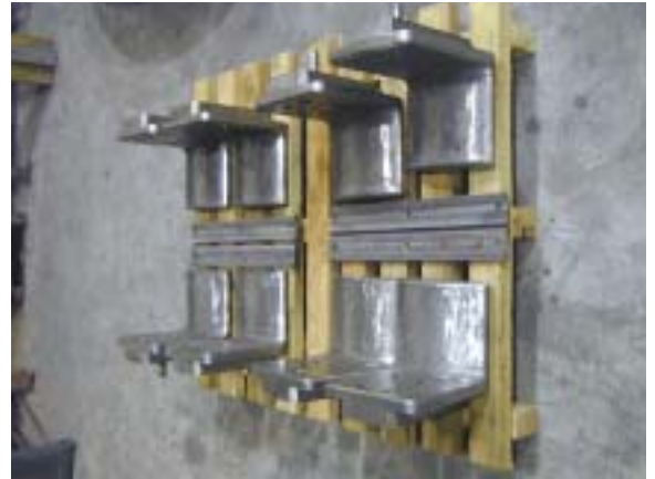
Segments with rough carbide coating
