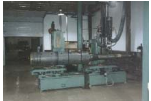
Mandrel segment shaft laser hardened bearing areas
