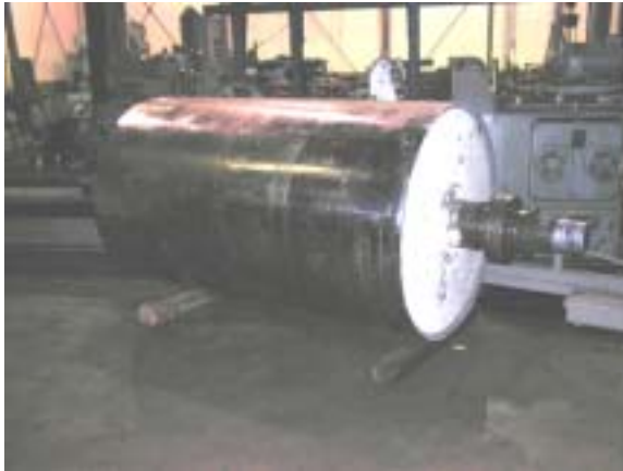
Mill roll awaiting carbide coating
