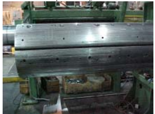
Damaged segment to be repaired
