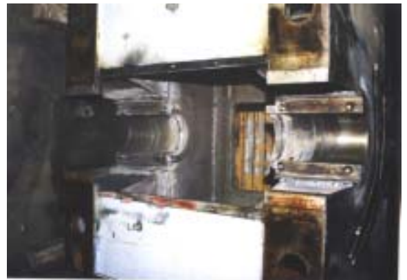
Steel slab grinder reworked bearing bores
