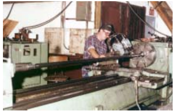
Flattening roll carbide coated, ground & polish finish to 8 - 10 RA. Life 2-3 months vs 3-5 days with chrome
