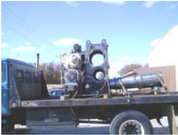
Expanding mandrel sleeve and housing. Repaired bearing bores on housing, laser hardened taper bore in sleeve
