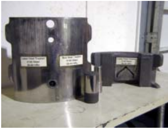
Laser hardened mandrel segment- OD and wedge (samples)
