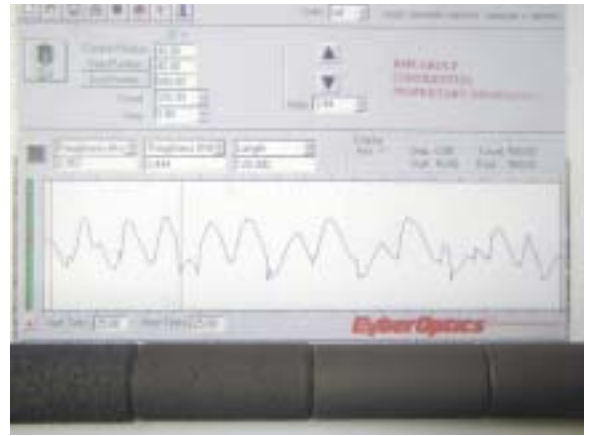
Various textured surfaces and example of laser roughness measurement report
