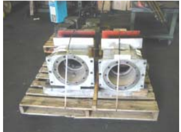
Trimmer housing, steel mill repaired bearing bores
