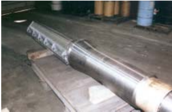
Mandrel shaft, laser hardened on taper area Carbide coating on segment area
