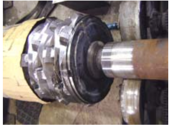
Large granulator shaft replaced broken end
