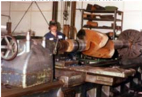
Mixer paddles machined bearing and seal areas
