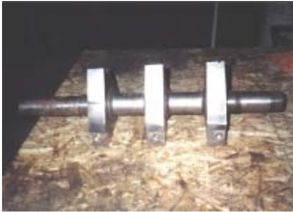
Small granulator rotor repaired bearing areas
