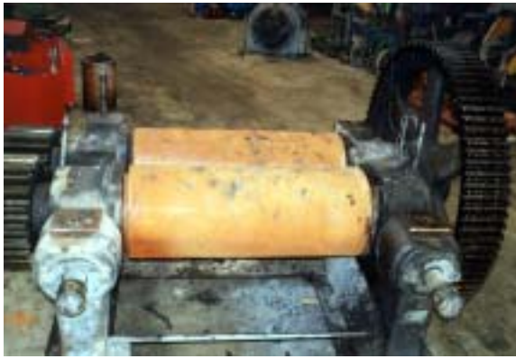
rubber mill being disassembled for total rebuild
