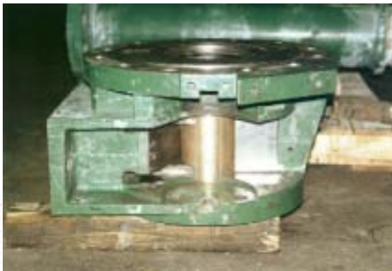
Extruder feed box rebuilt to specifications
