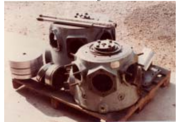
air compressor rods, cylinder and pistons totally rebuilt to specifications
