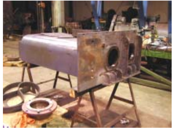
Large housing rebuilt bearing bores
