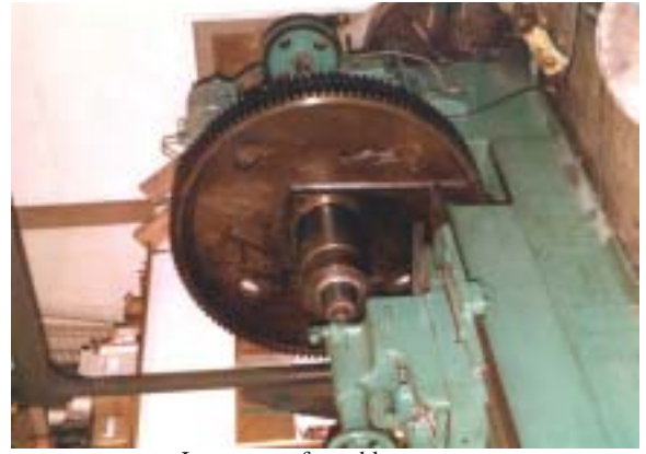
Large gear for rubber press rework bearing area
