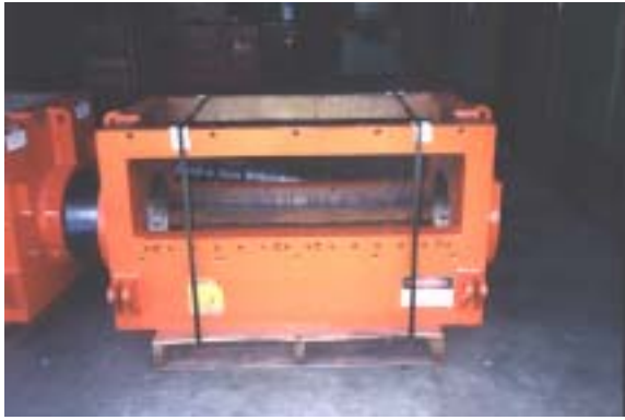
Granulator frame rebuilt bearing bores and knife bed
