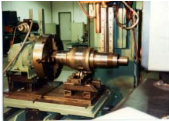
Shaft laser hardened tapered bearing area to 58-60Rc
