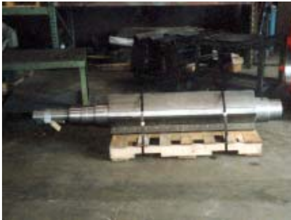
large granulator rotor reworked bearing areas and knife bed area
