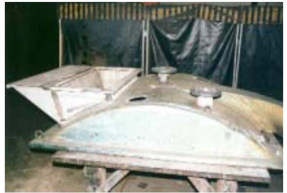
Stainless steel lid modified for large mixer
