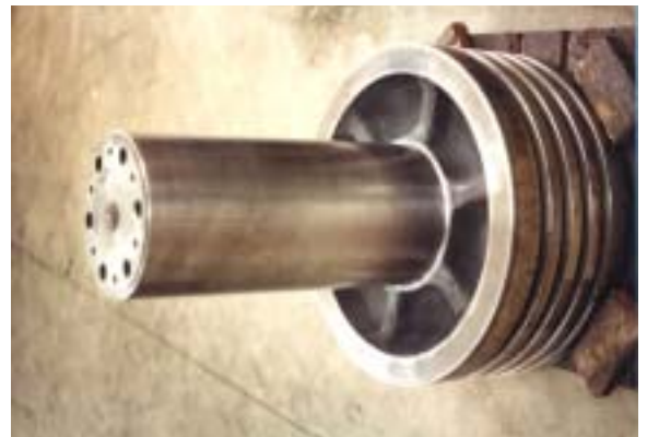
24-inch hydraulic piston ram area built up with 420SS and ground to size
