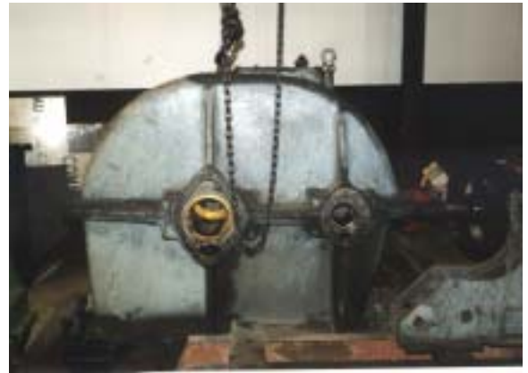
Gear box rebuilt bearing bores and shaft seal areas
