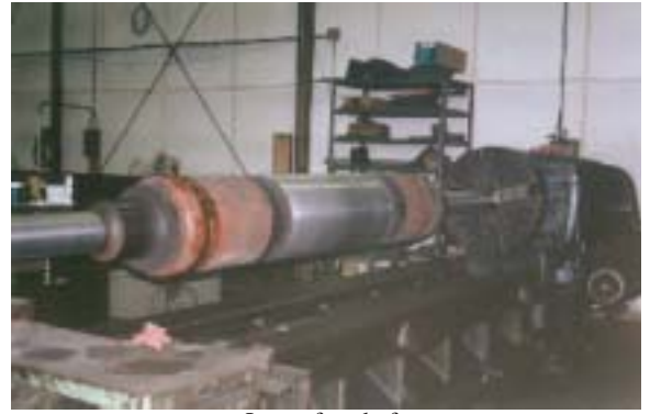
Large fan shaft repaired bearing areas and center section
