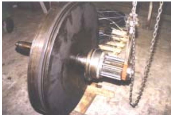
Punch press flywheel and shaft repaired to specification
