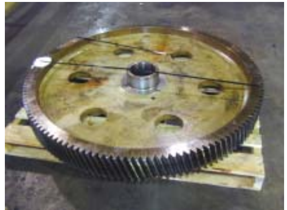
Large gear replaced four teeth and recut
