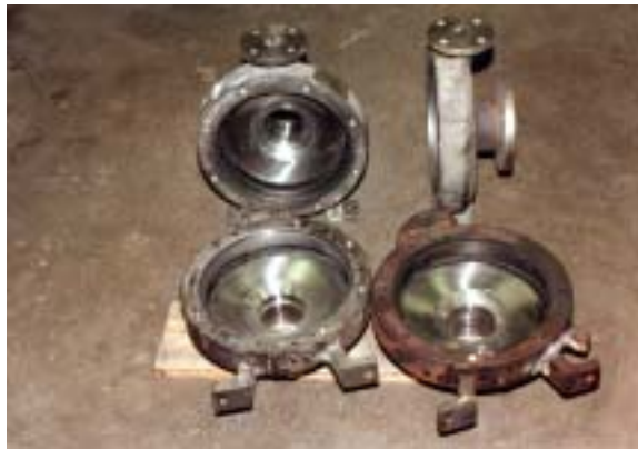
Pump housings rebuilt by welding and thermal sprayed coatings
