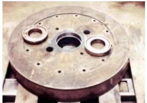
Press flywheel repaired bearing bores
