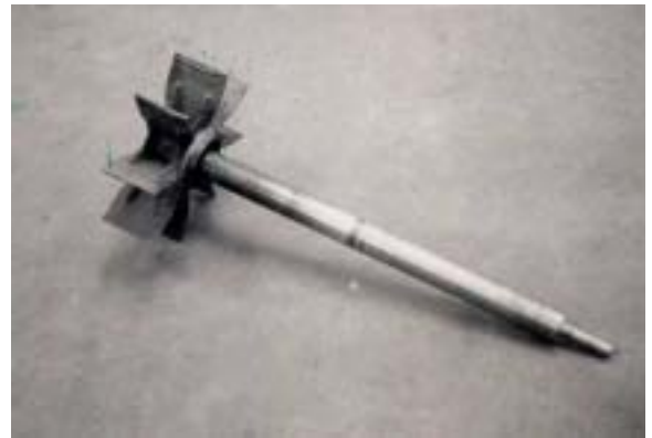
Material handling fan repaired bearing areas and fan blades
