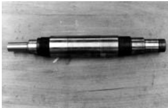
Machine tool spindle repaired bearing and seal areas
