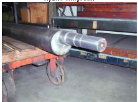
Eccentric shaft for foundry shaker repaired bearings and seal area
