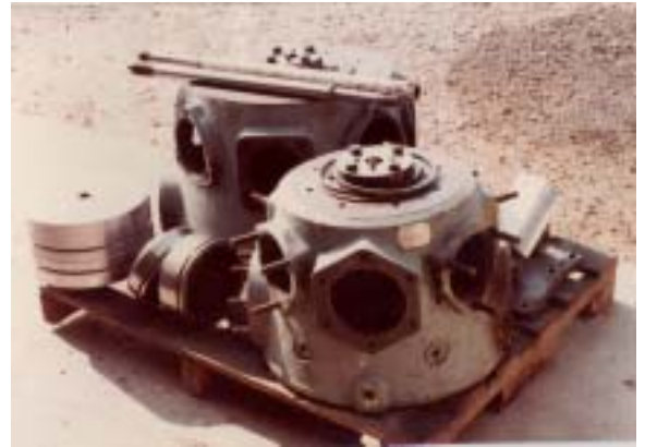
Air compressor rods, cylinder, and pistons totally rebuilt
