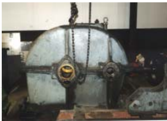
Gearbox rebuilt bearing bores and shaft seal area
