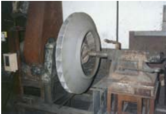
48-inch fan coated with .030 420SS for wear resistance
