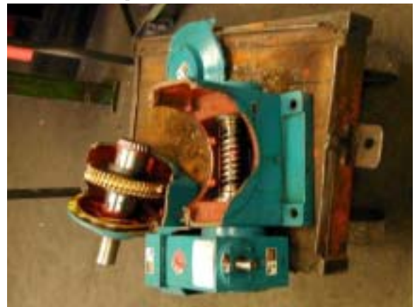
Broken gear box repaired (foreign unit)
