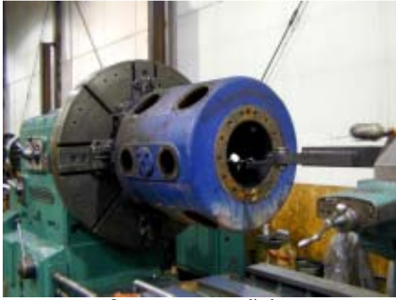
Large compressor cylinder rebuilt ID with 420SS
