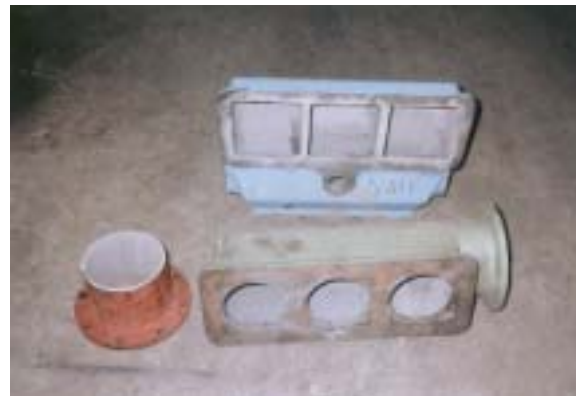
Diesal parts carbide coated to improve wear resistance to sand
