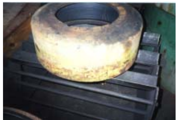
Brake drum for off-highway truck built up ID with 420SS and finished
