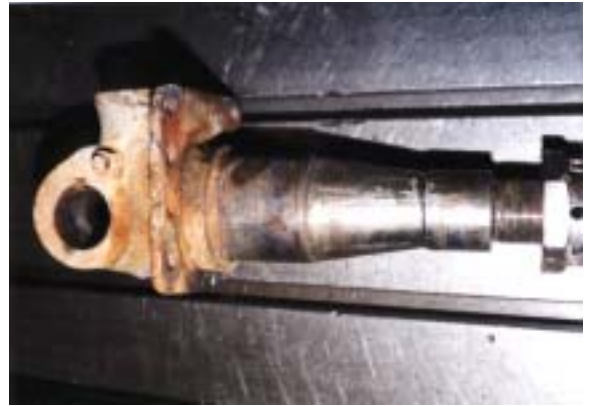
Front spindle for large quarry truck repaired bearing areas
