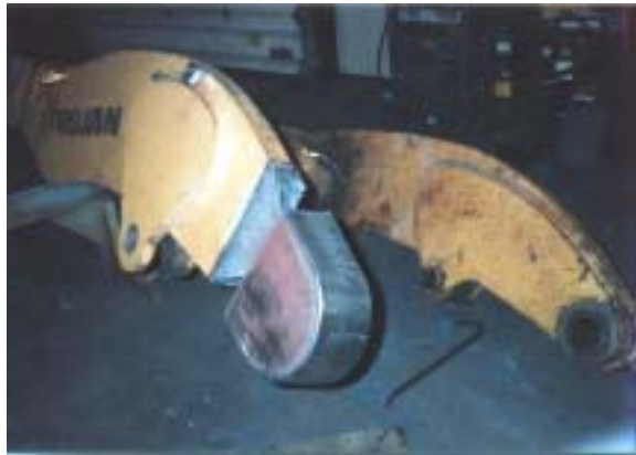
Loader frame replaced broken end
