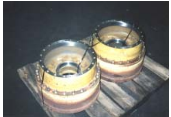
Hubs for large loader reworked bearings and seal areas
