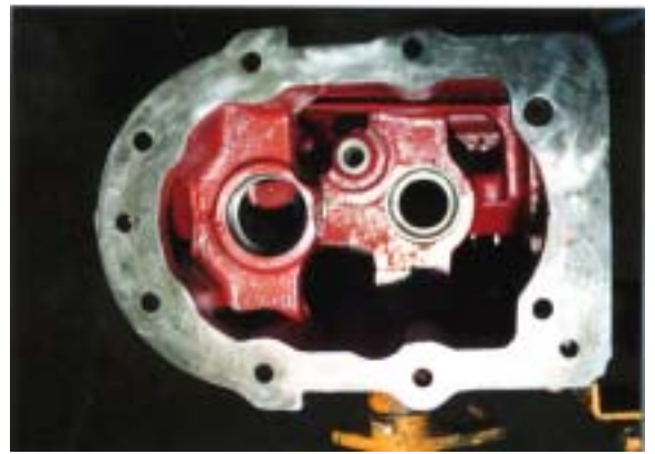
Transmission bearing repaired bore
