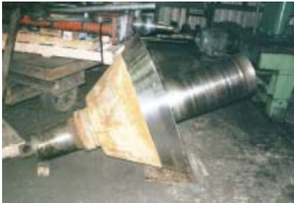
Crusher cone repaired bearing areas
