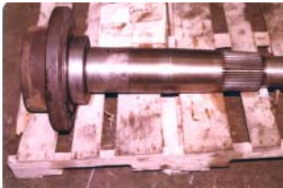
Off-highway equipment repaired drive axel bearing and seal areas
