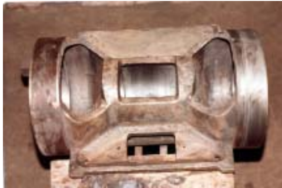
Crane swinger housing repaired bearing seats
