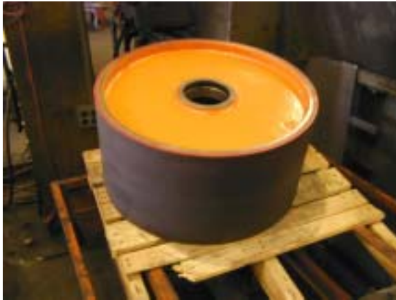
Roller drum repaired bearing area and turned OD
