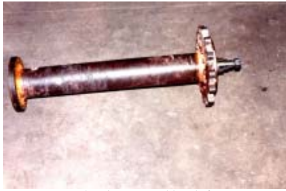
Elevating scraper drive shaft repaired and added new end
