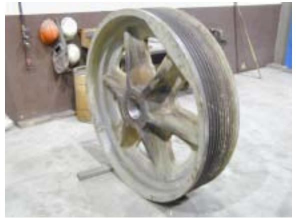
Large sheave for quarry repaired bore area
