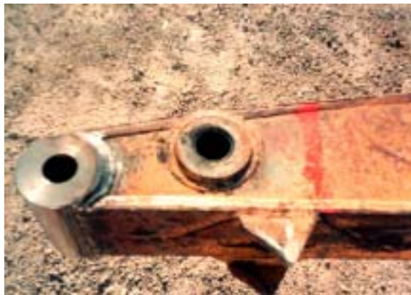
Excavator arm replaced end
